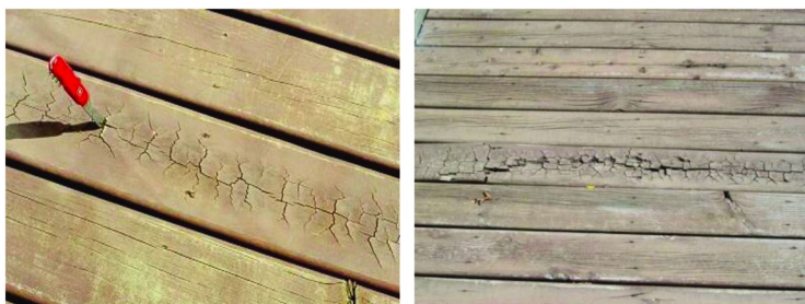
Figure 8. A CCA-treated pine deck board with exposed juvenile-wood surface after 5-years (left) and after 18-years (right) of direct outdoor exposure in Wisconsin. (Courtesy of J. Winandy with permission.)
