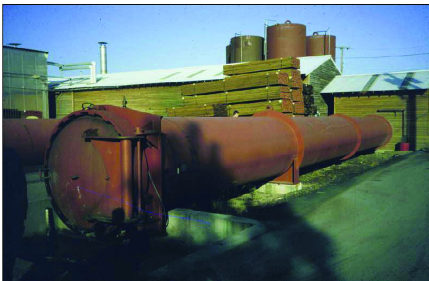
Figure 2. Example of a wood treating vessel or retort.
