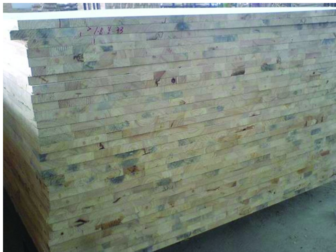
Figure 6. Rubberwood treated inefficiently with resultant blue stains.
